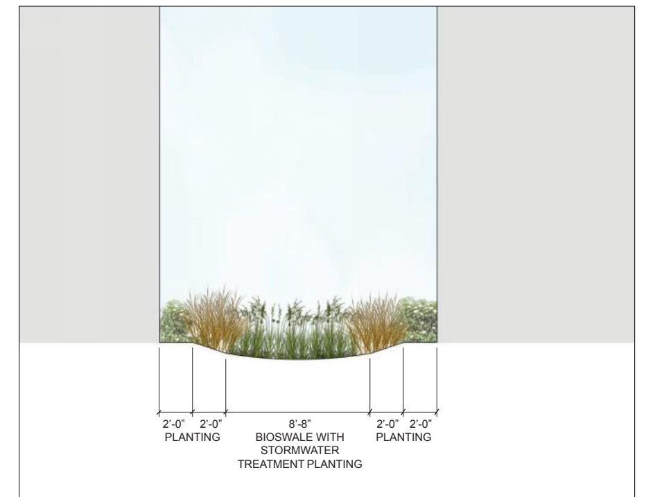
SECTION G-G: BIOSWALE AT HOUSING LOT
